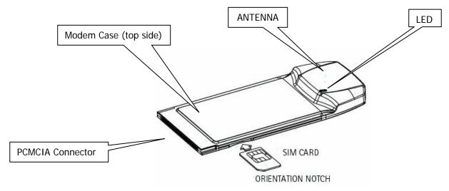
2. Insert the modem into the PC card slot of your PC. Windows reads the information from the Modem and installs drivers for each function of your UMTS Merlin.
